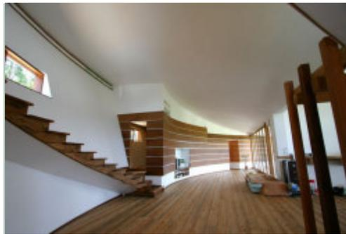
Shikkui natural lime plaster from Japan was used on the curving, unbroken interior walls of this residence.
